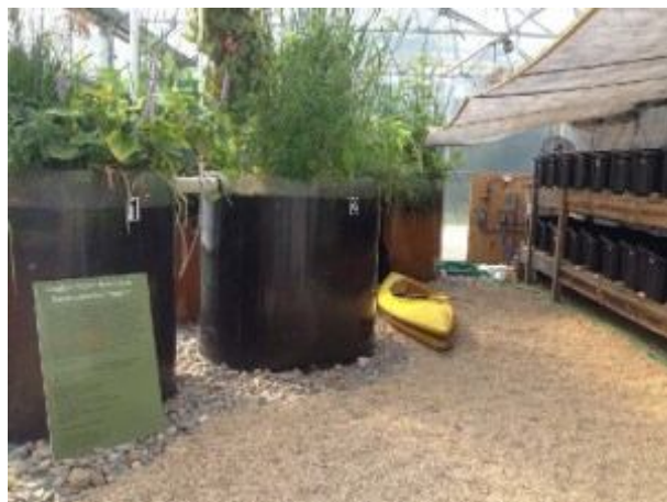
Aquatic cells and Myco-Reactors inside of greenhouse
